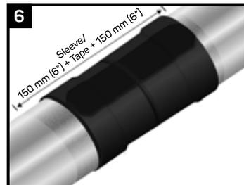
Do not sweep blast these types of field joint coatings.
