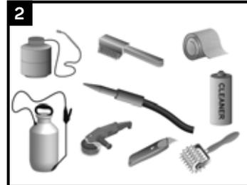
Appropriate tools for surface abrasion and preparation (wire brush/power wire brush or grit blaster, abrasive paper (60-80 grit), knife, lint free rags, approved solvent and high volume water sprayer, perforation tool, standard safety equipment: latex and leather gloves, safety glasses, hard hat, etc.
