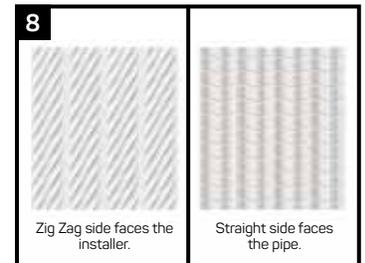
SCG must be wrapped onto the field joint in the correct orientation as shown above. The "Zig Zag" side of the SCG is the side that must face outward towards the installer. (Zig Zag Out). The straight side of the SCG is the side that must contact the pipe's surface.
