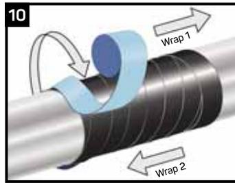
Apply the compression film **immediately** after the Scar-Guard has been installed. Apply the compression film in the same spiral direction as the SCG with a 50% overlap. Start min. 150 mm (6") beyond the outer edge of the SCG, pulling firmly during application to compress all SCG layers together, and end 150 mm (6") past the SCG on the opposite edge. The compression film must be installed with a minimum of 4 layers thick (2 passes at 50% overlap). Apply compression film with high tension.
