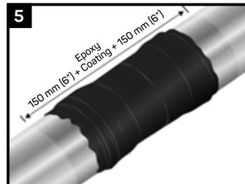
1. Sweep blast a minimum of 150mm (6") past the FJC edges on both sides. Sweep blasting should result in a 25 to 75 microns (1 to 3 mil) profile. Be careful not to cause a holiday when sweep blasting. With approval from the coating manufacturer, sweep blast the entire epoxy girth weld coating resulting in a 25 to 75 microns (1 to 3 mil) profile.
