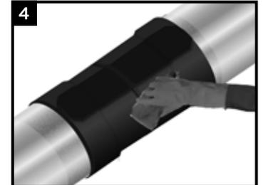
Perform an SSPC SP1 solvent cleaning. Remove all visible signs of oil, grease, dust, dirt or other surface contaminants; clean the FJC and the adjacent pipe coating with a solvent cleanser. To determine the width of the area to be cleaned refer to step 5 or step 6.
