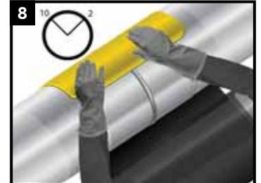
Centre the sleeve over the joint so that the sleeve overlaps between the 10 and 2 o'clock positions. Press the underlap firmly into place.
