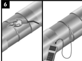
Pre-heat the joint area to the minimum of 65°C (150°F). Using a temperature measuring device, ensure that the correct temperature is reached on the steel and at least 50mm (2") on each side of the sleeve.
