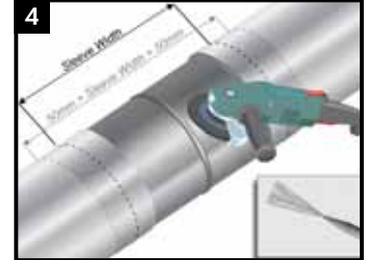
Ensure that the pipe is dry before cleaning. Using a power wire brush, abrade the pipe to a minimum of St3/SP3 (abrasive blast to Sa2.5/SP10 recommended). Lightly abrade the pipe coating adjacent to the cutback area to a distance of 50mm (2") beyond each end of the sleeve width.
