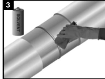
Ensure that the mainline coating edges are beveled to 30°. If there is the presence of oil, grease, or other surface contaminants; clean the exposed steel and adjacent pipe coating with a solvent cleanser.
