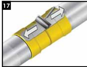
Continue the procedure by also firmly rolling the closure with long horizontal strokes from the weld outwards.
